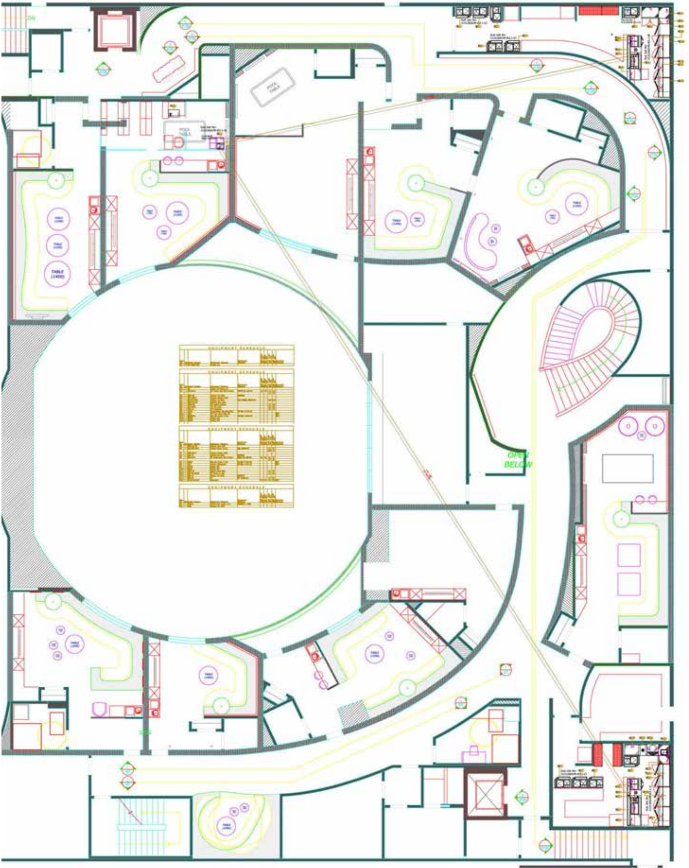
The drawing depicts two full service bars serving to PDRs with multiple bar trolleys to serve independently, and central soda reserve feeding carbonated beverages to the service bars.
